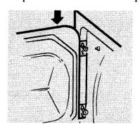
7 Remove the remaining screws from the side of the opening from which the door was removed. With these screws secure each hinge at the bottom.
